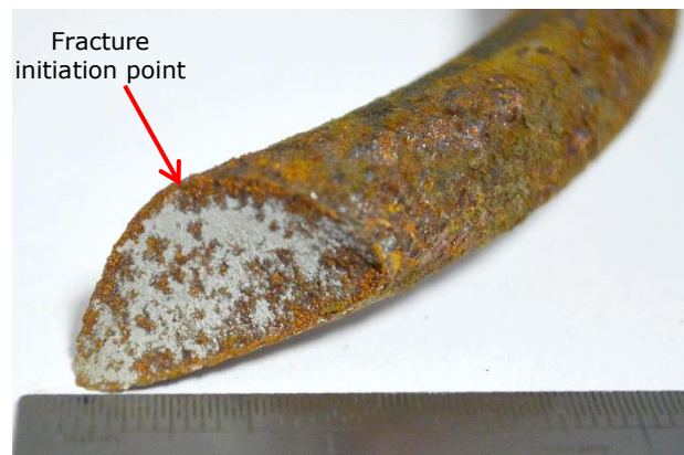
Figure 4. The fracture face with the location of the initiation point indicated.
