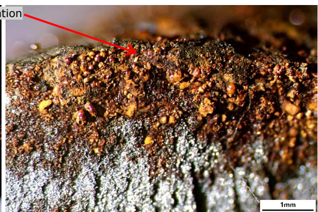
Figure 6. The region of fracture initiation, spoiled by corrosion.
