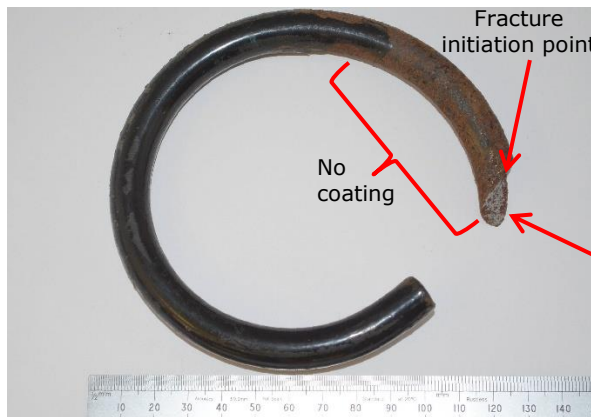
Figure 1. The received portion of the failed helical spring.
