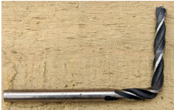
Figure 1. The failed drill bit.
