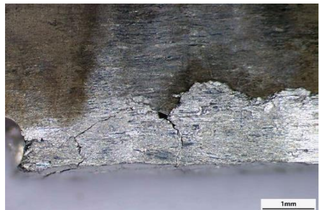
Figure 4. A higher magnification of the affected area on a blade.
