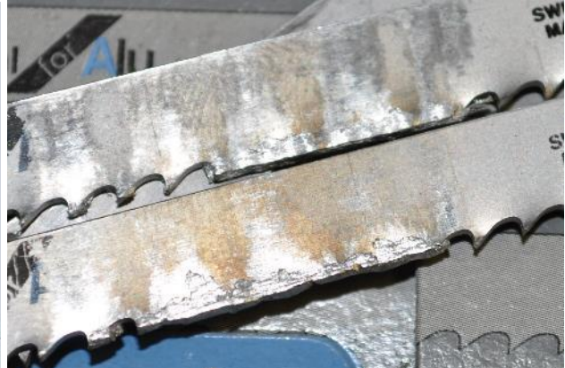
Figure 2. The affected areas of the jigsaw blades.
